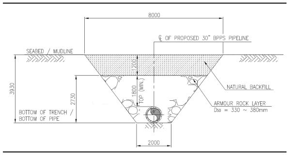
Figure 3.6 Trench Design (Type F)
