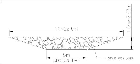
Figure 3.2 Trench Design (Type B)
